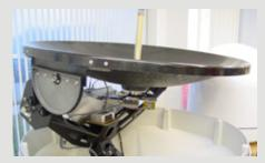
Many mobile satellite communications antennas rely on the KVH DSP-3000 for accurate pointing and stabilisation.
